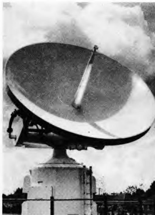
Sl. 30. Meteorološki radar (Plessey 43S)
